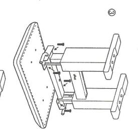
Bolt bench frame to the bottom of the bench top as shown and tighten the bolts securely.
